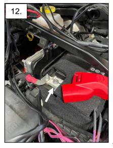
13. Next to the fuse block is a chassis ground. Using a 10mm socket, remove the nut & place the 3/8" ring terminal on the black wire to the chassis ground.
